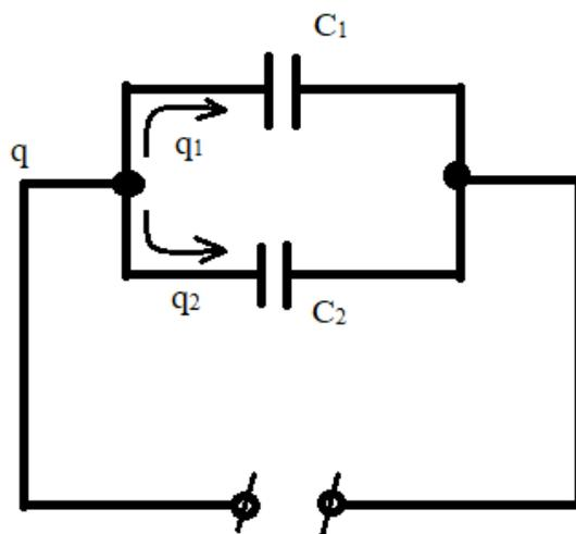
$$\begin{aligned}q_1 + q_2 &= q \\U_1 = \frac{q_1}{C_1} &= U_2 = \frac{q_2}{C_2} \\q_2 &= \frac{q_1 \cdot C_2}{C_1} \\q &= q_1 \frac{C_1 + C_2}{C_1} \\q_1 &= \frac{q \cdot C_1}{C_1 + C_2} \\q_1 &= \frac{2,3 \cdot 10^{-6} \cdot 10 \cdot 10^{-6}}{11,5 \cdot 10^{-6}} = 2 \cdot 10^{-6} \text{ Кл} = 2 \text{ мкКл}\end{aligned}$$
